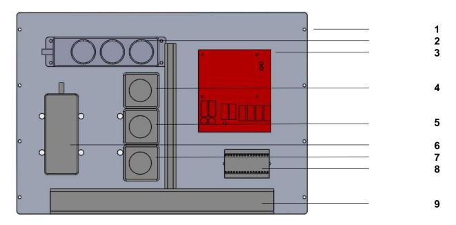
1 Base plate control unit cubeONE 2 3times power socket, current power, 230VAC - max. 4A 3 Basic board - BLP Reading spot 230VAC, switched over control panel 4 5 power socket 230VAC, switched by working position 6 power supply 12VDC 7 power socket 230VAC switched, max. 2A 8 external connection 9 cable guide
