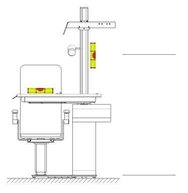
Correct adjustment of the refraction unit
